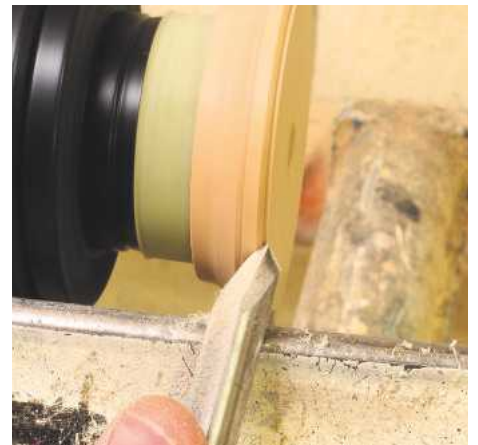
▲ Pic.15 Because he is working on side grain the bead must be turned the opposite way than usual on spindle work, the tool starting at the bottom of the profile and being worked towards the top
